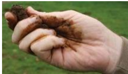
Figure A-4. Step 4 of the ribbon test.
